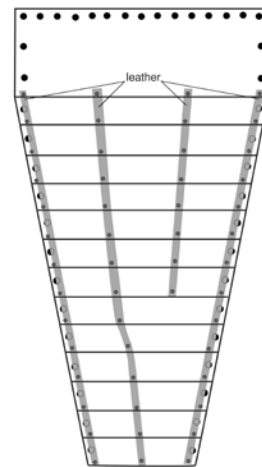
Simplified diagram illustrating the internal leathering of an armguard, with the leathers attached to the interior of each lame with a rivet. The larger circles are apertures for the attachment of a removable, padded lining. (Drawing © M.C. Bishop)
